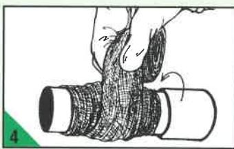
4. Using entire roll, wrap **Python Wrap** approximately 2" above repair area, working it directly over the leak patch. Continue wrapping and extend **Python Wrap** approximately 2" below repair area.
