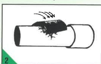
2. Remove the adhesive backing from the leak patch and apply directly over the break or hole.
