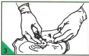
3. Wearing enclosed gloves, (gloves are most effective when applied to dry hands) tear open foil pouch at the notched area. Remove **Python Wrap** from the foil pouch and soak in warm water for 20 seconds.
