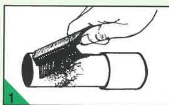
1. Clean and roughen area to be repaired. Pipes and hoses should be shut down prior to repair.
