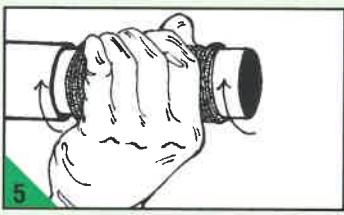
5. Squeeze and mold **Python Wrap** in the direction of wrap, removing excess water, while spreading resin until tacky to touch. Wait 30 minutes before reapplying pressure to the system.
